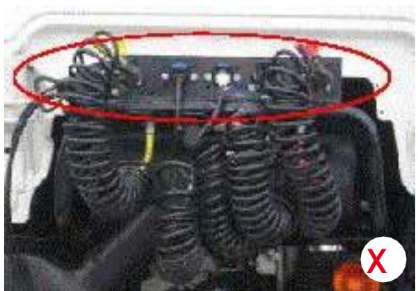
Air lines and cables are not in the right place.
