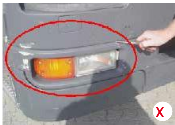
Scratched and broken bumper
