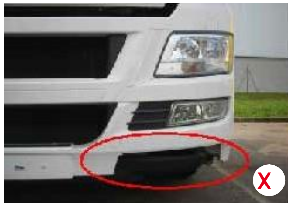
Missing bumper corner
